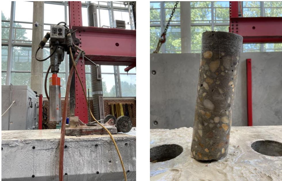
Figure B.6: Girder top flange coring.
