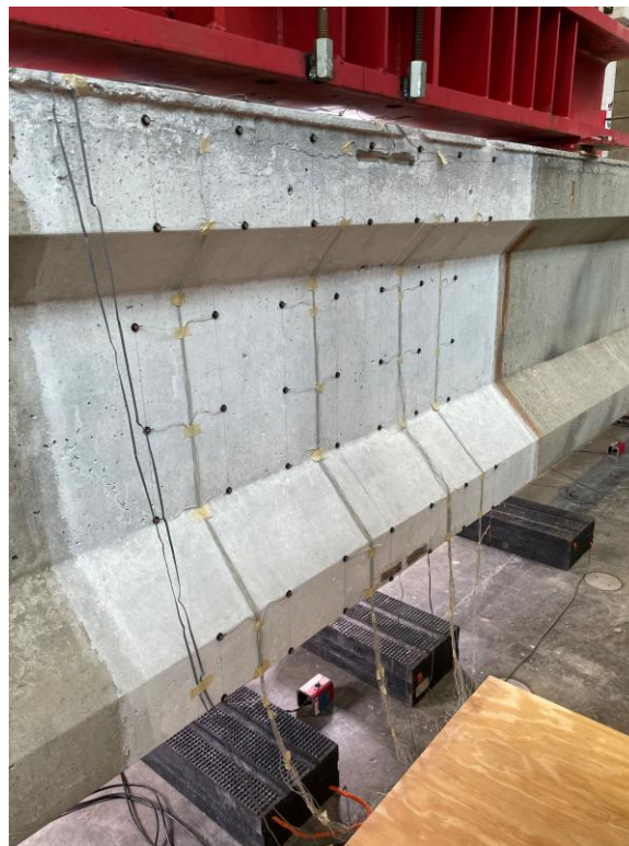
Figure B.24: Optical LED grid at midspan.
