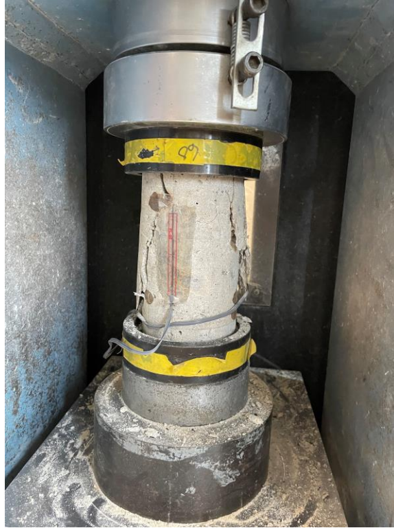
Figure B.19: Deck core failure around steel reinforcement.
