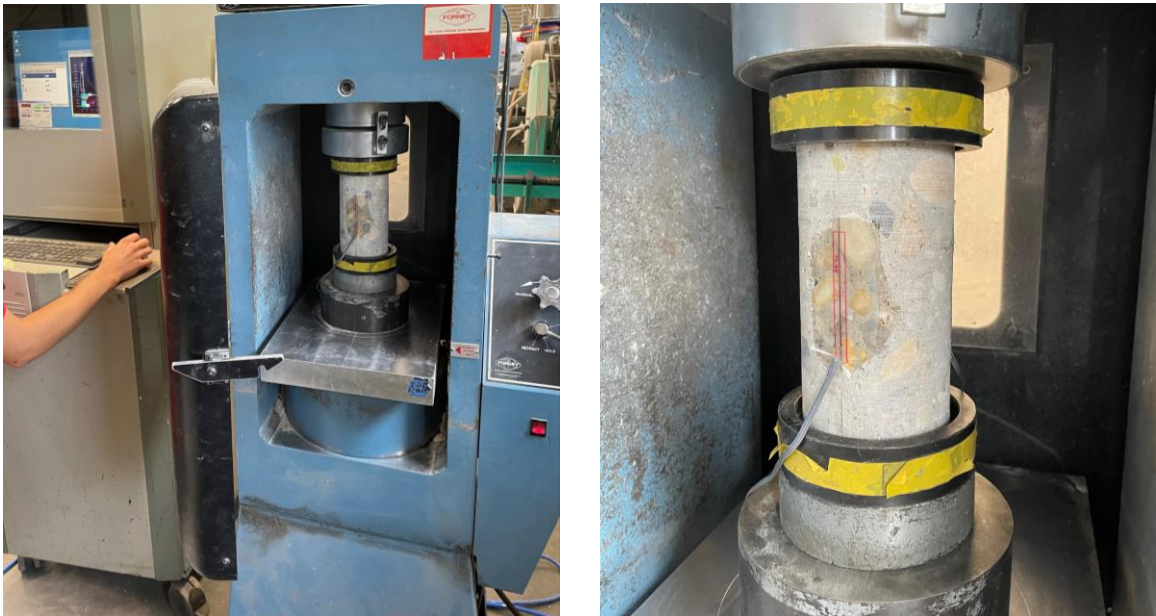
Figure B.8: Core compression testing.
