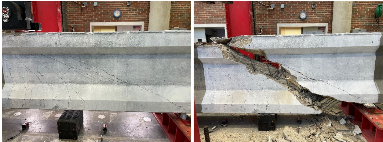
a) Final Load Stage : 310 kips
