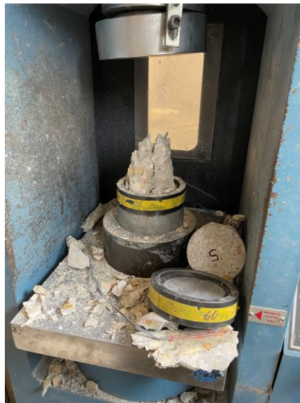
Figure B.11: Typical failure of core from BTE1.
